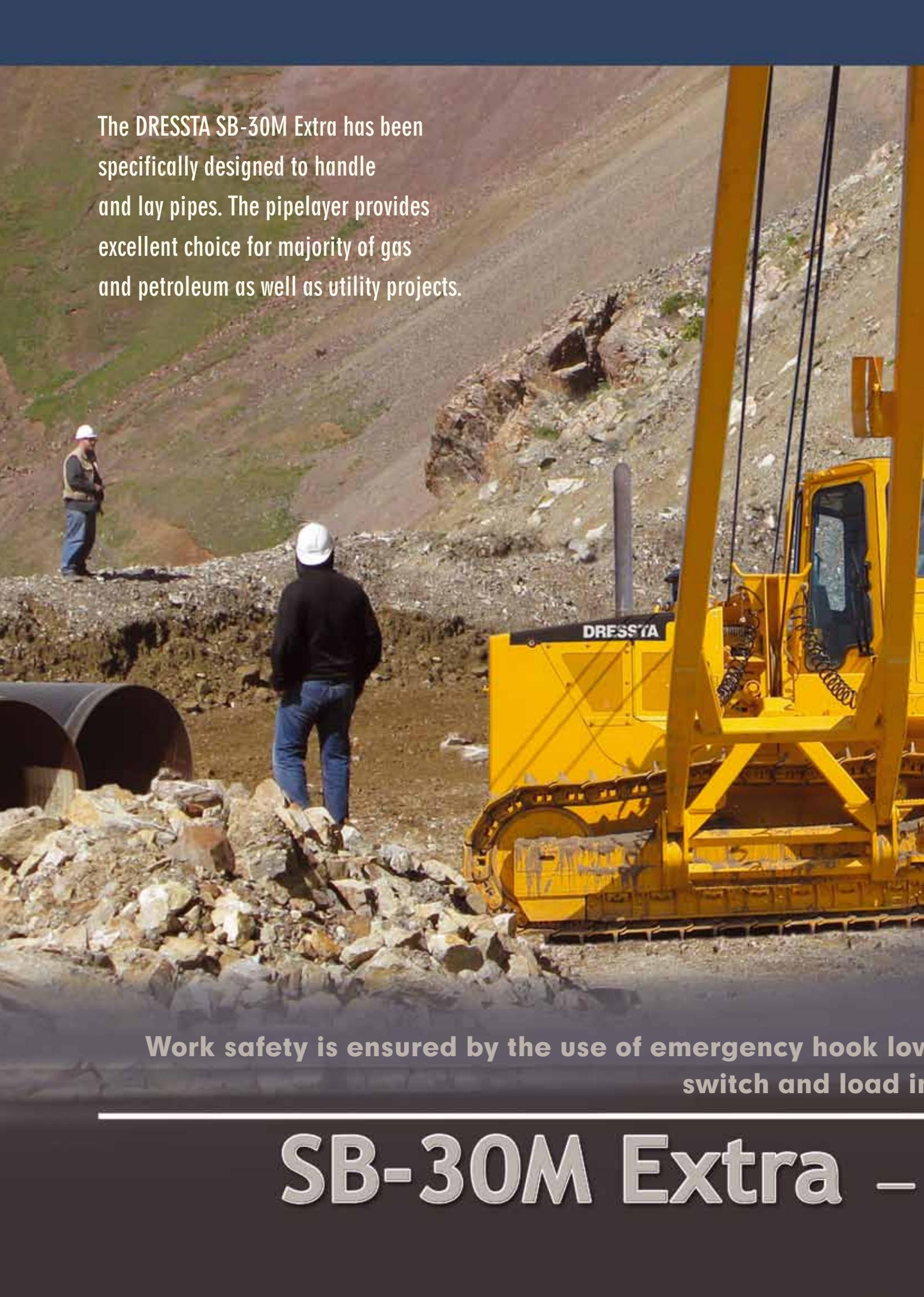
The DRESSTA SB-30M Extra has been specifically designed to handle and lay pipes. The pipelayer provides excellent choice for majority of gas and petroleum as well as utility projects.
