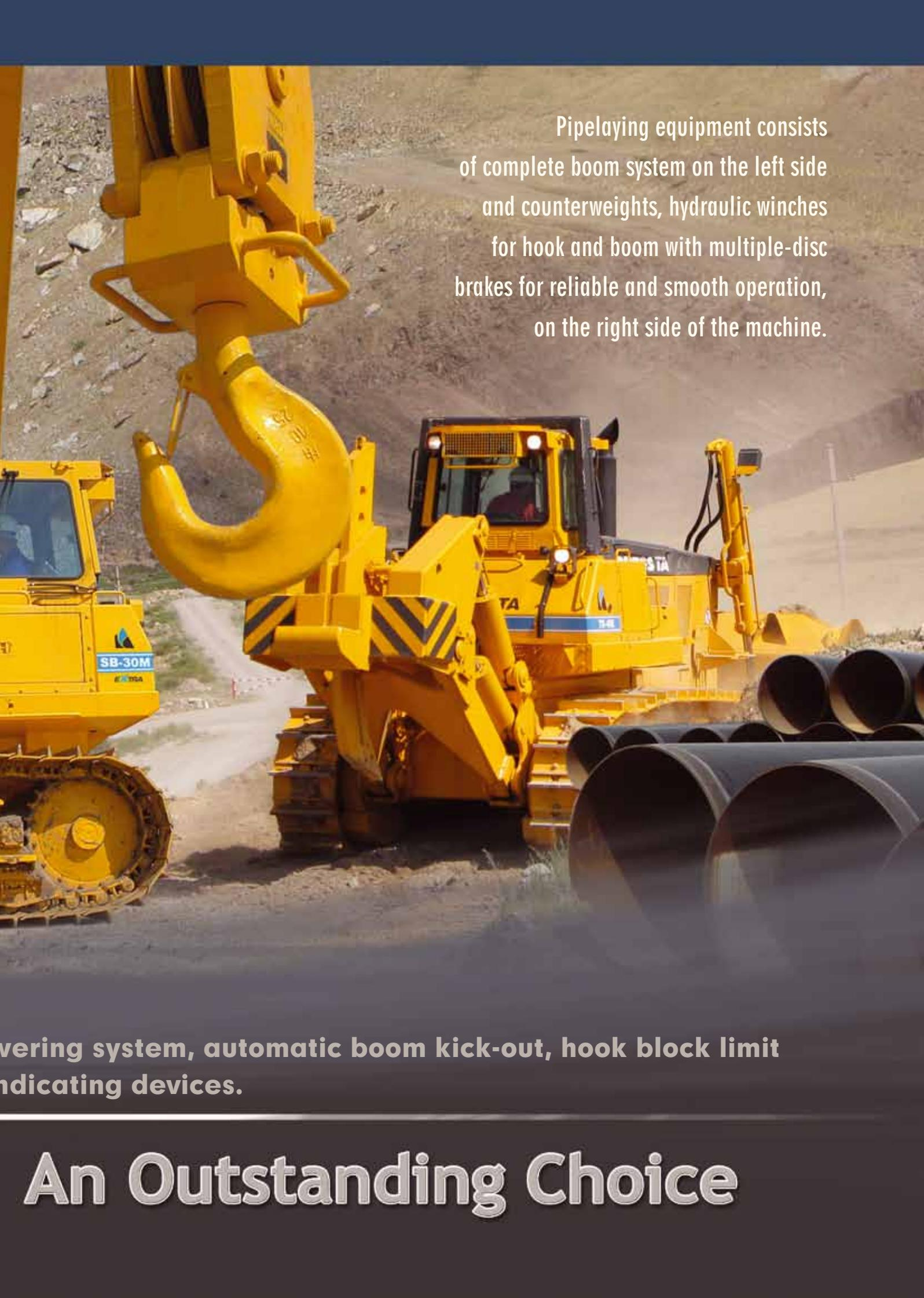
Pipelaying equipment consists of complete boom system on the left side and counterweights, hydraulic winches for hook and boom with multiple-disc brakes for reliable and smooth operation, on the right side of the machine.
