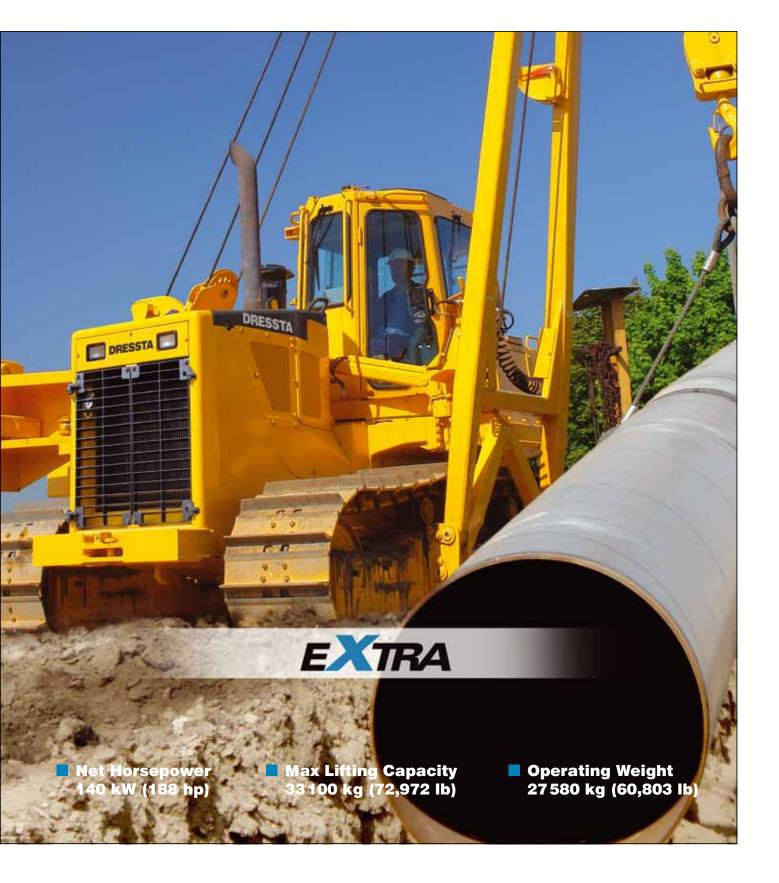
The DRESSTA SB-30M Extra has been specifically designed to handle and lay pipes. The pipelayer provides excellent choice for majority of gas and petroleum as well as utility projects.
