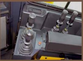
The two front levers control winches of the pipelaying equipment while the side levers actuate the counterweights that maintain the proper stability of the machine.
