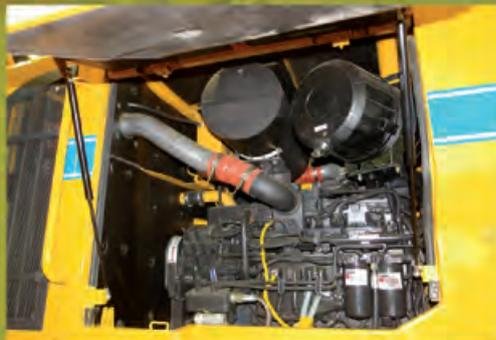
Cummins QSC8.3 engine meets EU Stage IIIA emissions standards. The QSC advanced electronics provide enhanced engine performance with higher torque and better throttle response at every rpm.
